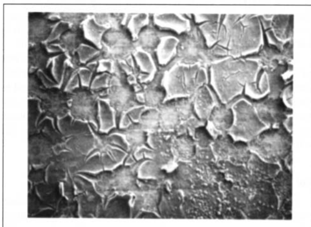
Figure 6. SEM calcium phosphate coating before cleaning.
